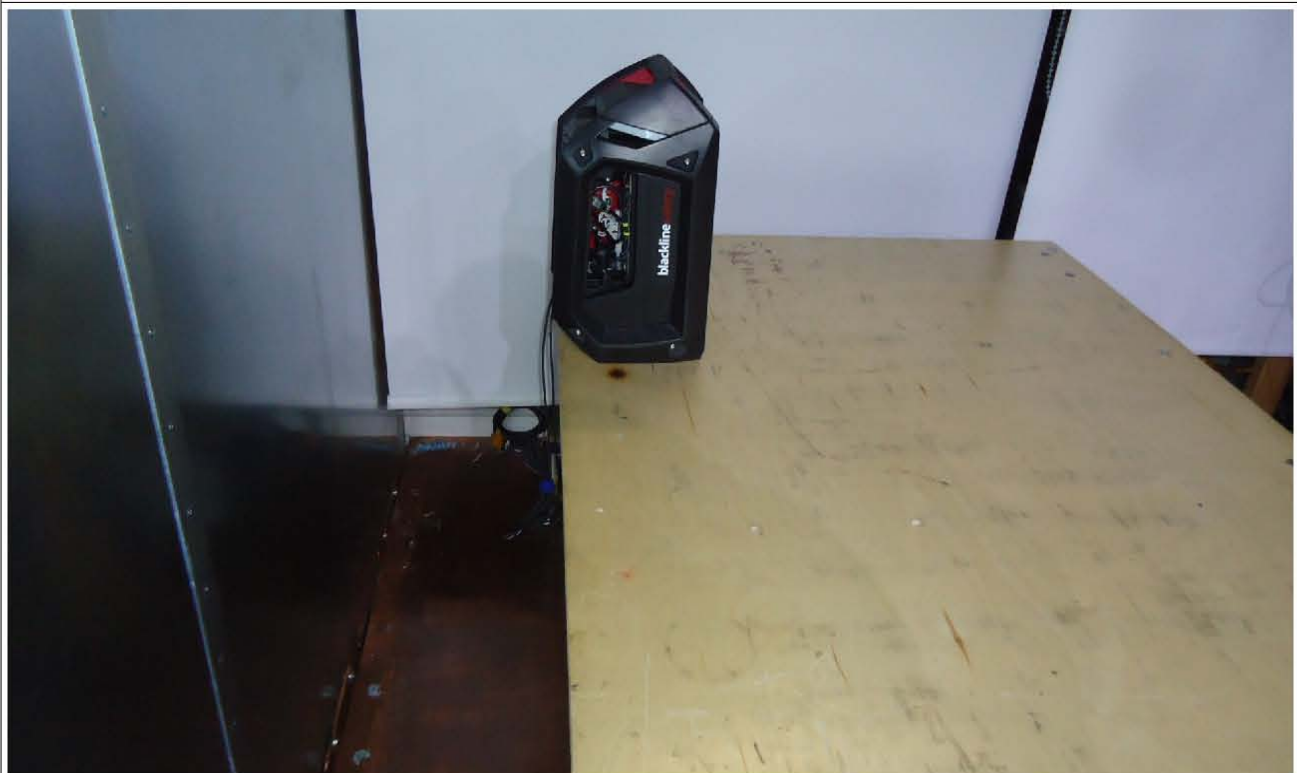
Figure 6.2 - Conducted Emission Test Setup - Side View
