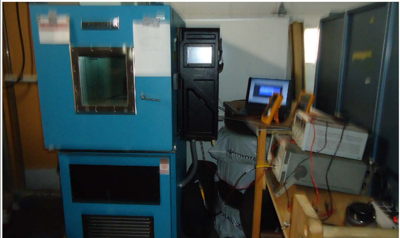
Figure 8.1 - Test Setup –Thermal Chamber and Power System
