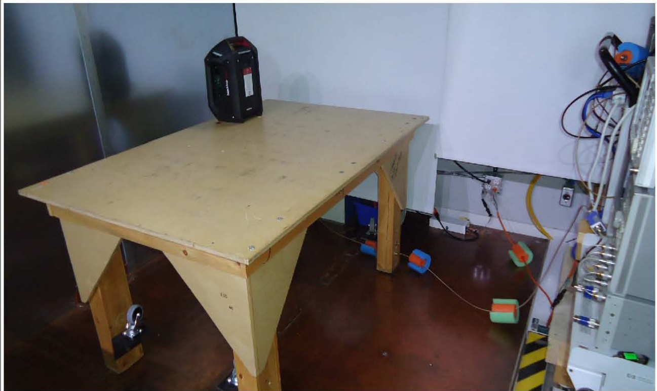
Figure 6.1 - Conducted Emission Test Setup - Front View
