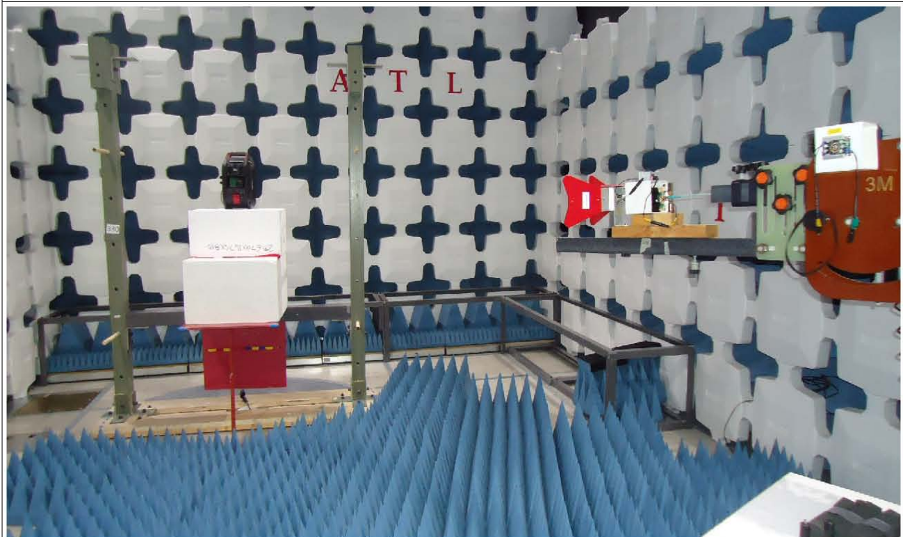
Figure 4.2 - Radiated Emission Test Setup - Side View
