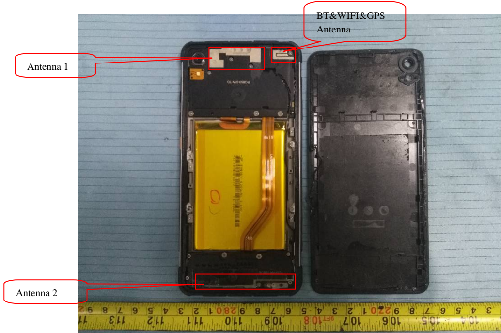
EUT – Cover off View 1
