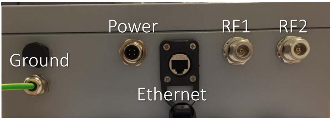
Connect the Ground wire to a solid ground accessible near the installation site.
