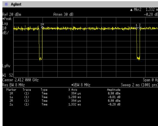
$$\text{Duty Cycle} = \text{Ton} / (\text{Ton} + \text{Toff}) = 1288[\mu\text{s}] / (1288[\mu\text{s}] + 44[\mu\text{s}]) = 96.7\%$$
