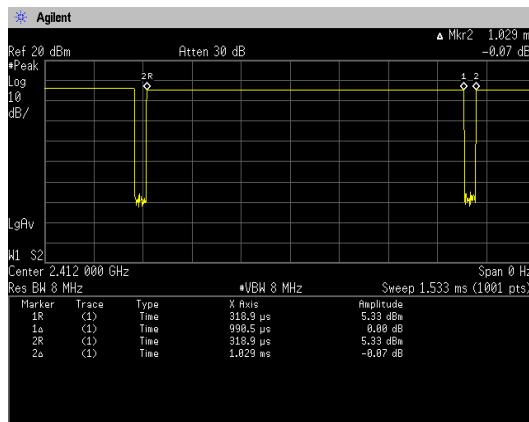
$$\text{Duty Cycle} = \text{Ton} / (\text{Ton} + \text{Toff}) = 990.5[\mu\text{s}] / (990.5[\mu\text{s}] + 38.5[\mu\text{s}]) = 96.26\%$$
