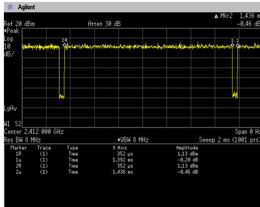
$$\text{Duty Cycle} = \text{Ton} / (\text{Ton} + \text{Toff}) = 1392[\mu\text{s}] / (1392[\mu\text{s}] + 44[\mu\text{s}]) = 96.94\%$$
