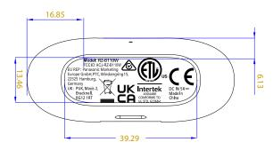
The marking information is located at the bottom of apparatus
