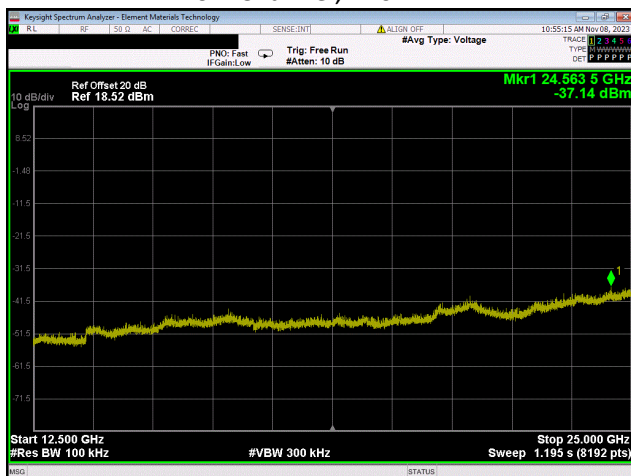
BLE/GFSK 1 Mbps Low Channel, 2402 MHz
