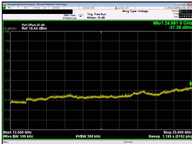
BLE/GFSK 2 Mbps Mid Channel, 2442 MHz
