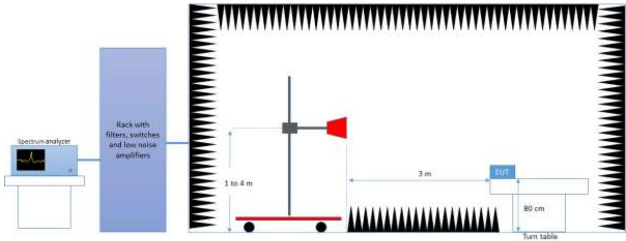
*Radiated Setup 18 GHz - 40 GHz*
