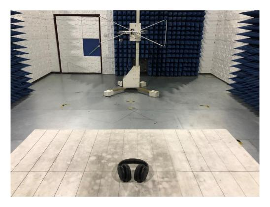
RADIATED EMISSION TEST SETUP ABOVE 1GHZ
