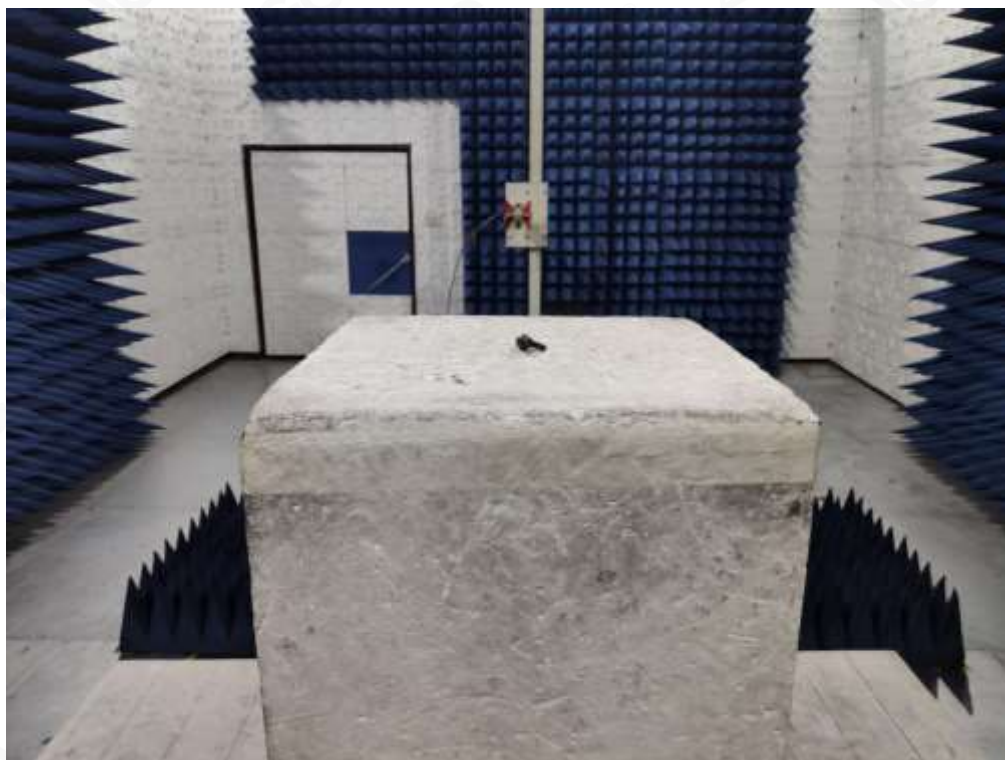
RADIATED EMISSION TEST SETUP ABOVE 1GHZ
