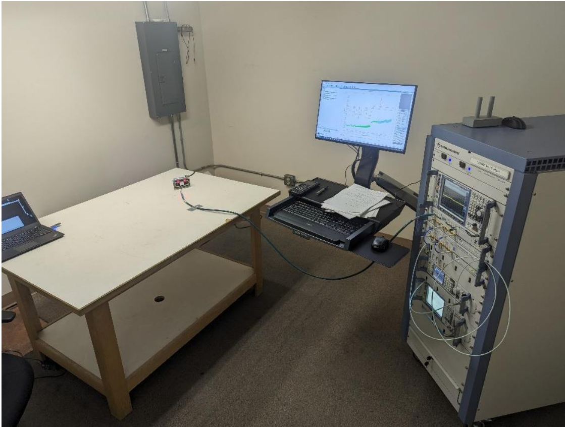
Photograph 8: Antenna Port Conducted Test Setup
