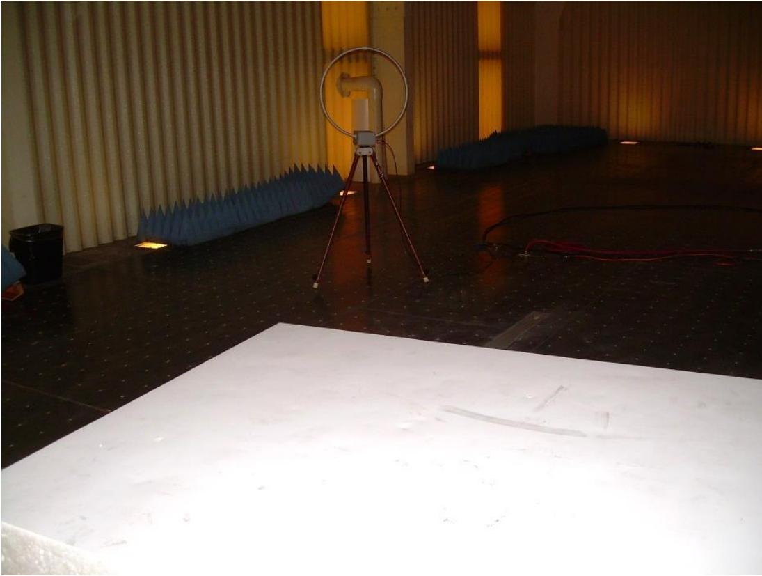
Photograph 11: Reference Photo of Test Setup for Emissions Below 30 MHz
