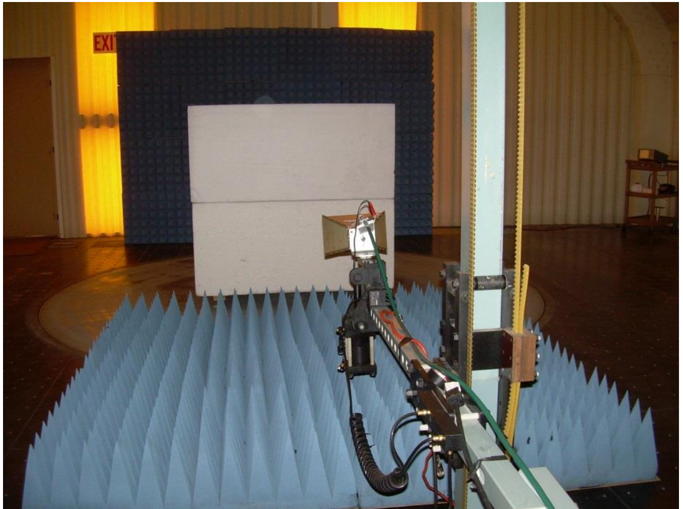
Photograph 13: Reference Photo of Test Setup for Emissions Above 1000 MHz
