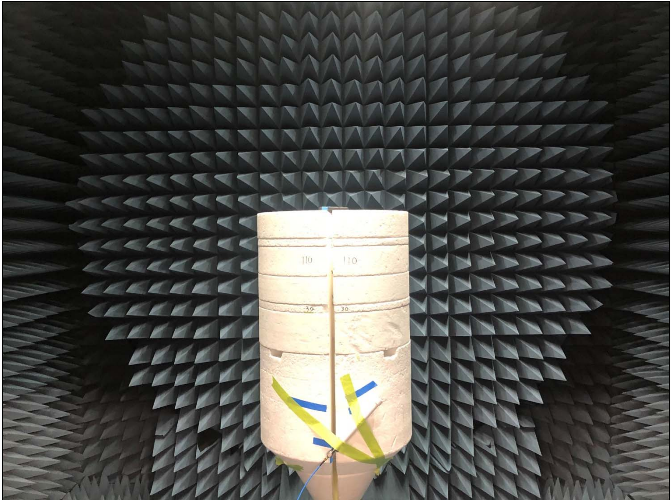
OTA EIRP Measurement, Test Setup, View 1
