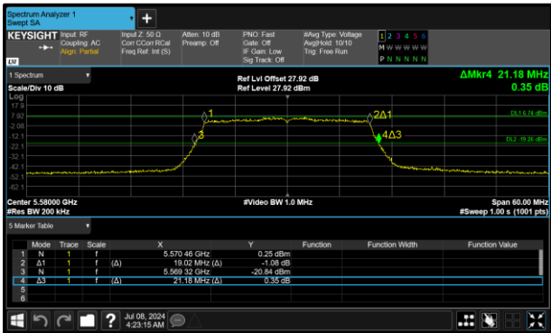
Figure 347 - 802.11ac VHT20 Maximum 99% OBW
