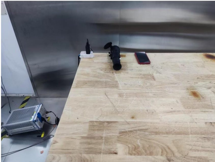
Conducted Emissions at AC Power Line (150kHz-30MHz)
