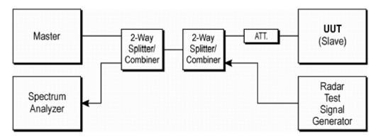
Figure 7-1. Test Setup
