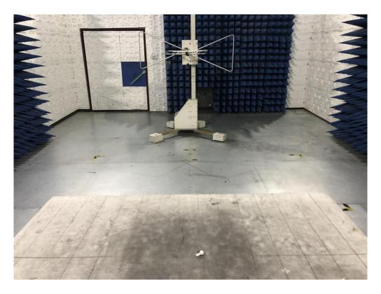
RADIATED EMISSION TEST SETUP ABOVE 1GHZ
