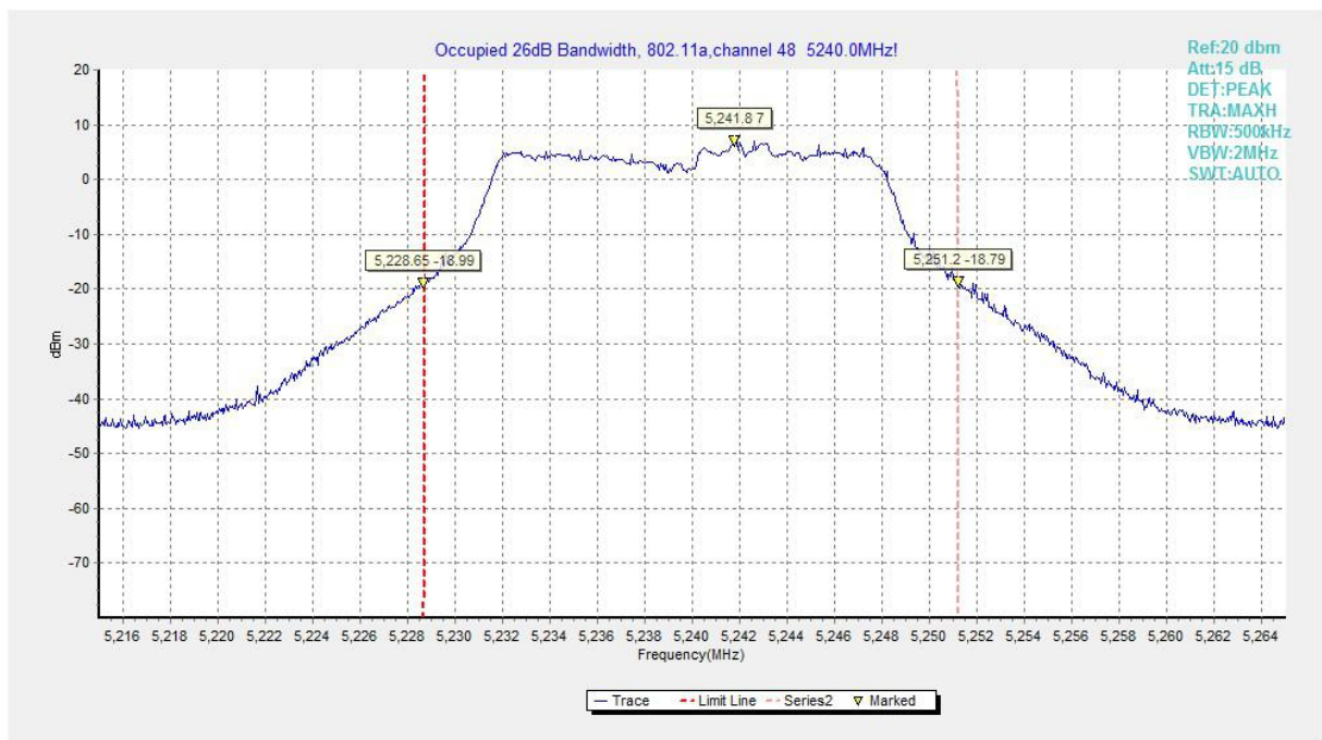
Fig.101 Occupied 26dB Bandwidth (802.11a, 5240MHz)
