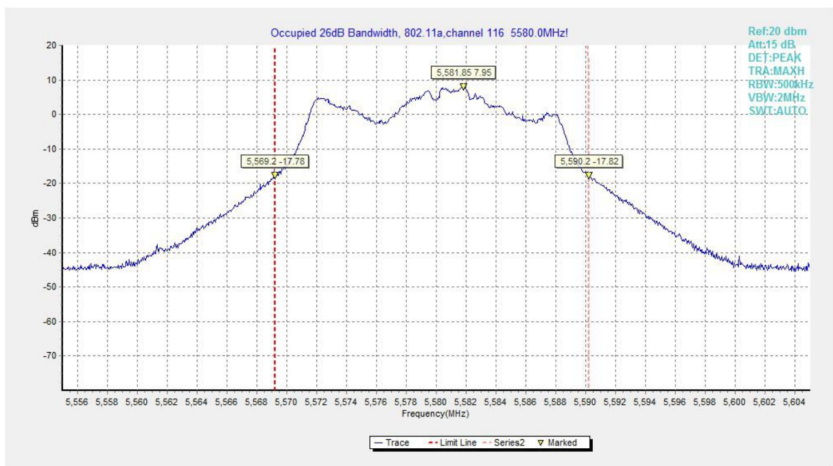
Fig.106 Occupied 26dB Bandwidth (802.11a, 5580MHz)
