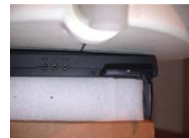
Figure 14.11 Body SAR Test Setup -- Lap Configuration --
