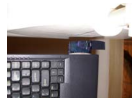
Figure 14.10 Body SAR Test Setup -- Bystander Configuration --
