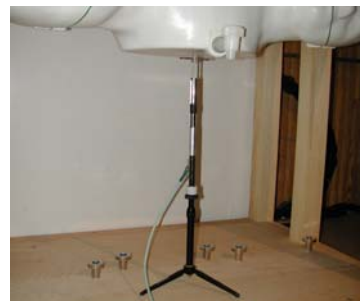
Figure 12.1 Dipole Validation Test Setup
