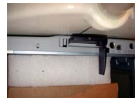
Figure 14.3 Body SAR Test Setup -- Lap Configuration --
