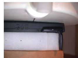
Figure 14.9 Body SAR Test Setup -- Lap Configuration --
