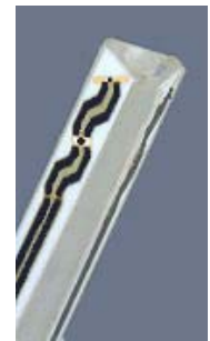
Figure 3.2 Probe Thick-Film Technique
