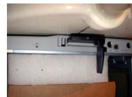
Figure 14.1 Body SAR Test Setup -- Lap Configuration --
