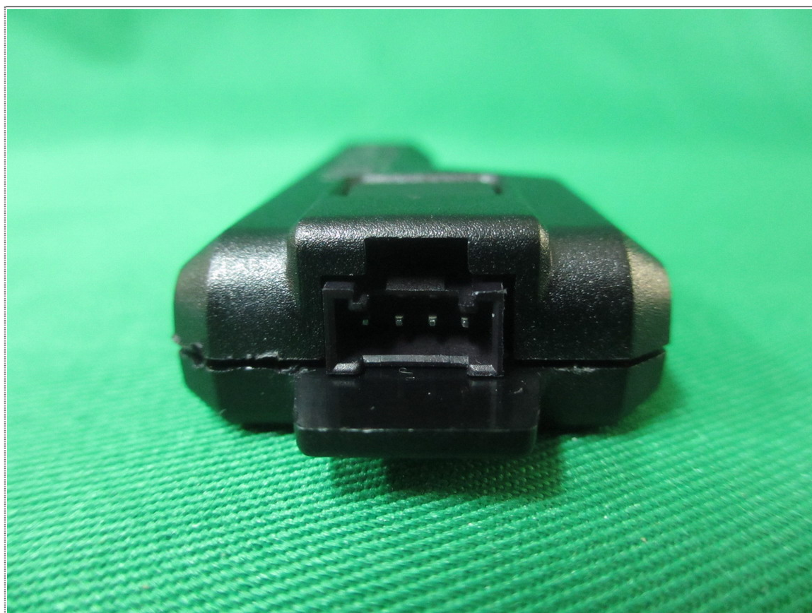
View of Power port
