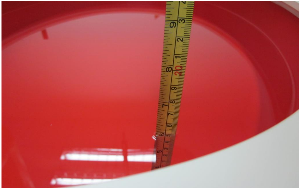
Figure 4.4: Liquid depth in the Flat Phantom
