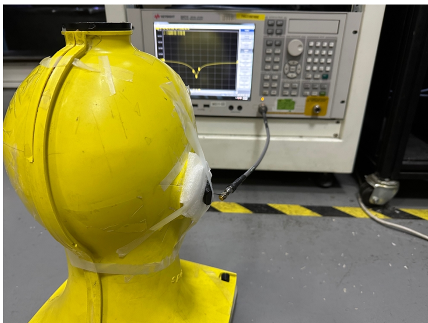
Beside Head Right Impedance Setup
