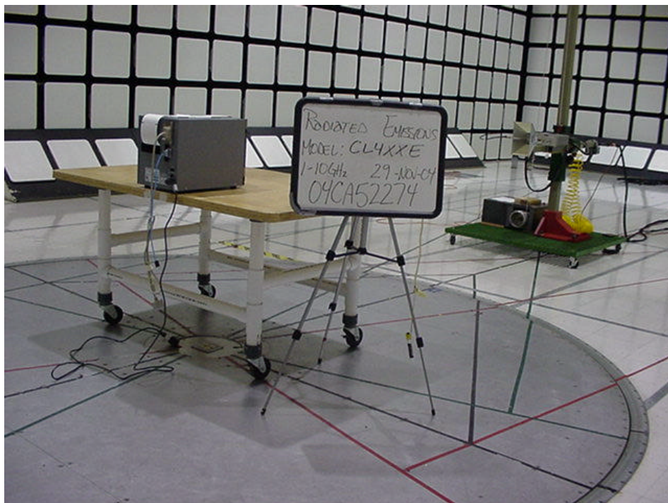
Radiated Emissions Test Setup 1-10 GHz
