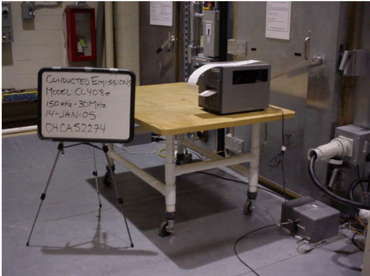
Conducted Emissions Test Setup
