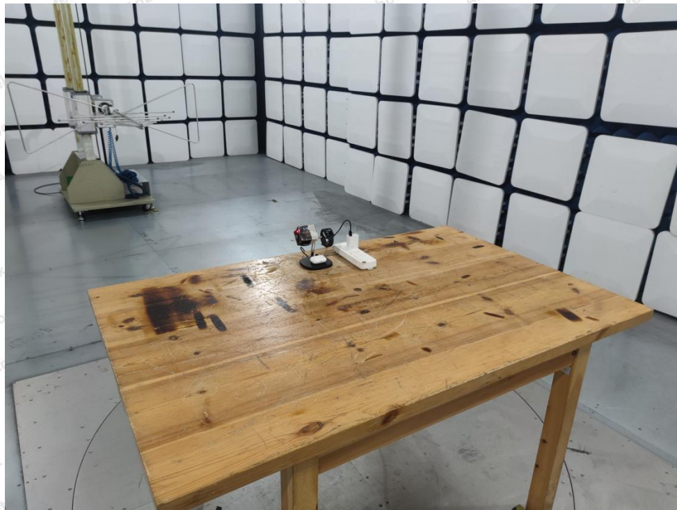
Photo of Radiation Emission Test
