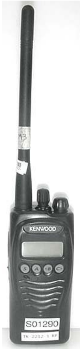
Front of DUT Whip Antenna (P/N: KRA-26M/M2/M3)
