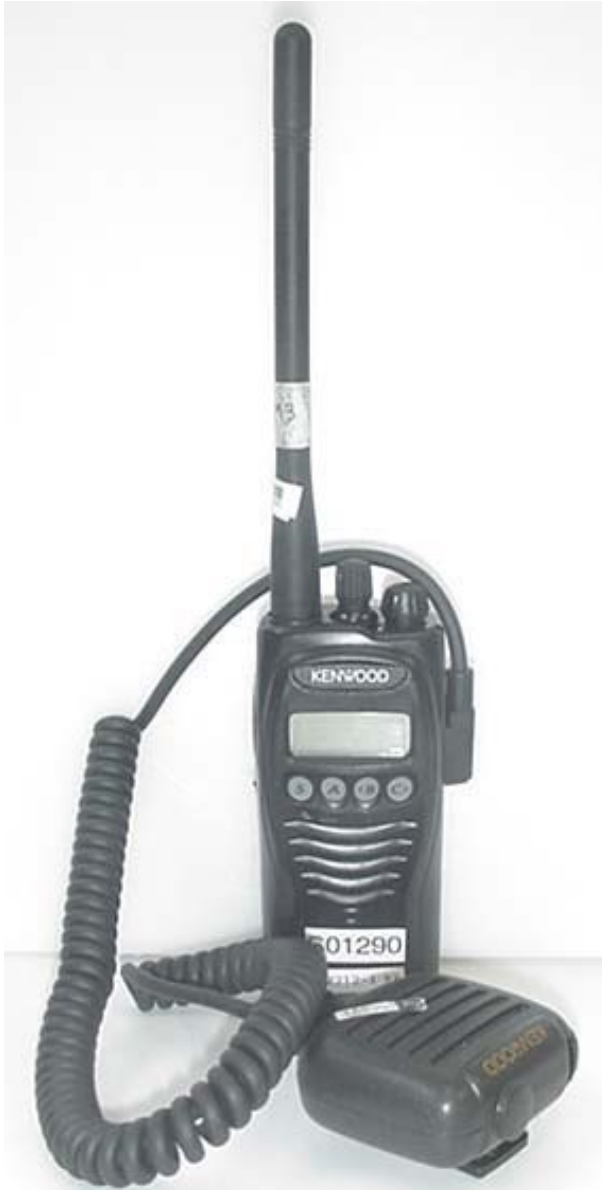
DUT with Speaker-Microphone Accessory (P/N: KMC-17)
