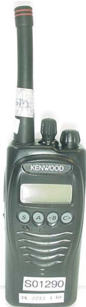
Front of DUT Stubby Antenna (P/N: KRA-16M)
