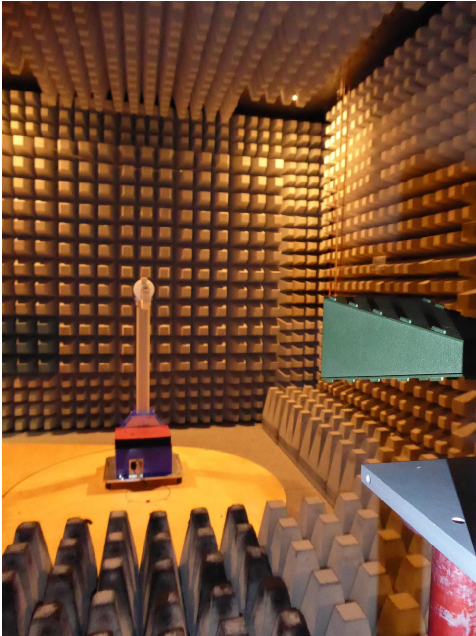
181323_SetRadC10.JPG: Test setup fully anechoic chamber; EVB-ANNA-B112C#143, 12 – 18 GHz
