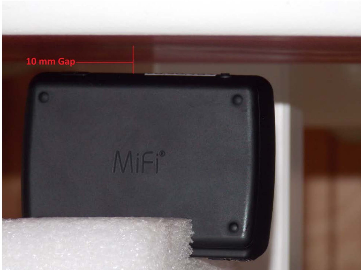
Test Position Side B 10 mm Gap
