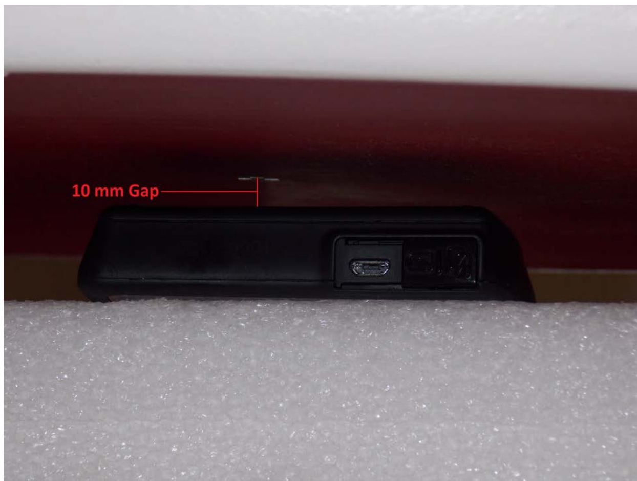
Test Position Side C 10 mm Gap
