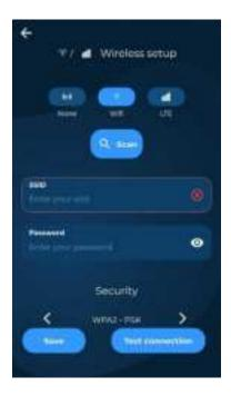
**SSID** : name of the WiFi to which you want to be connected to. Case sensitive
