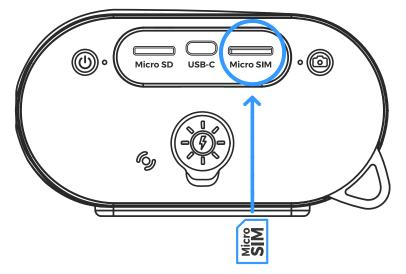
Inserting the SIM card: Metal contacts of the chip downwards, angle left to the bottom - see above.
