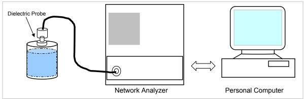
Set-up for liquid parameters check
