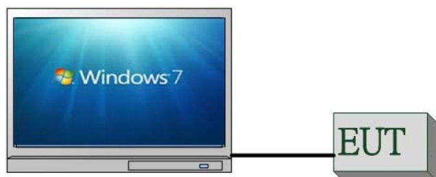
Fig. 2-1 Conducted (Antenna Port) Emission Configuration
