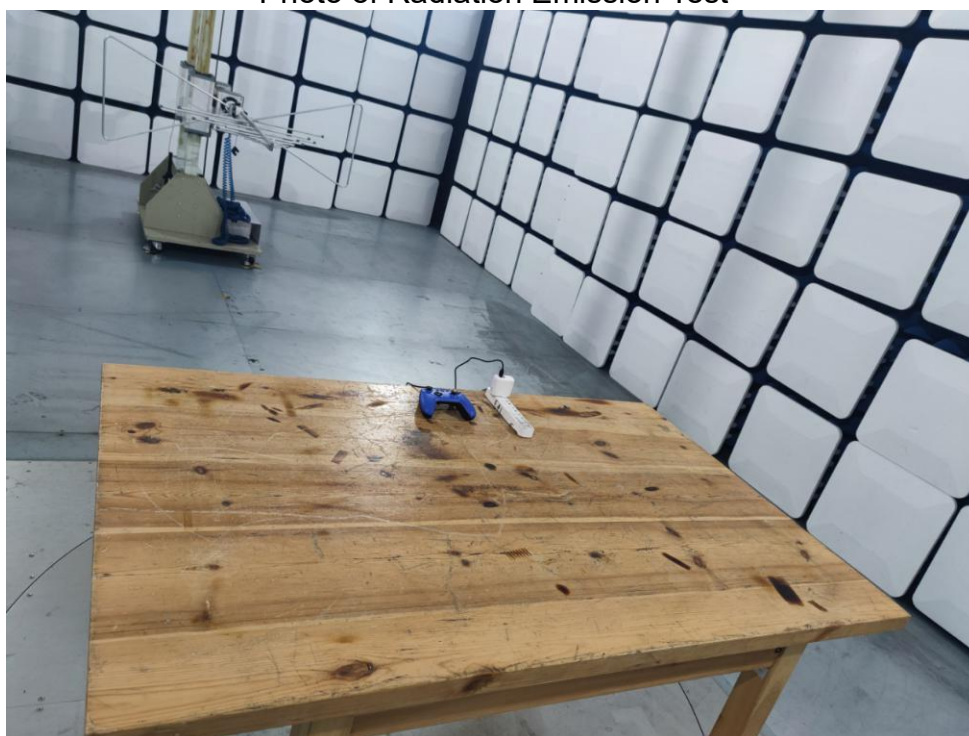
Photo of Radiation Emission Test
