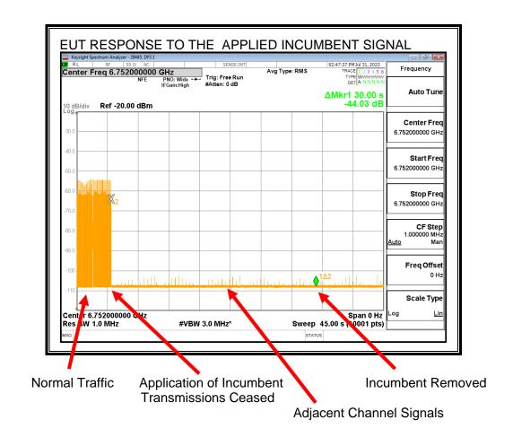
When the EUT detects the Incumbent AWGN Signal it switches to channel 1 and all signals on the test channel cease. Observable transmissions during the monitoring period are from the new adjacent channel to which the EUT has switched.
