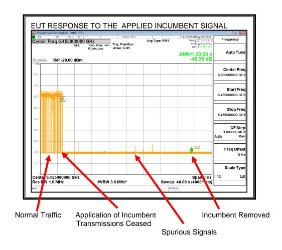
When the EUT detects the Incumbent AWGN Signal it switches channels and all signals with the exception of spurious signals on the test channel cease.
