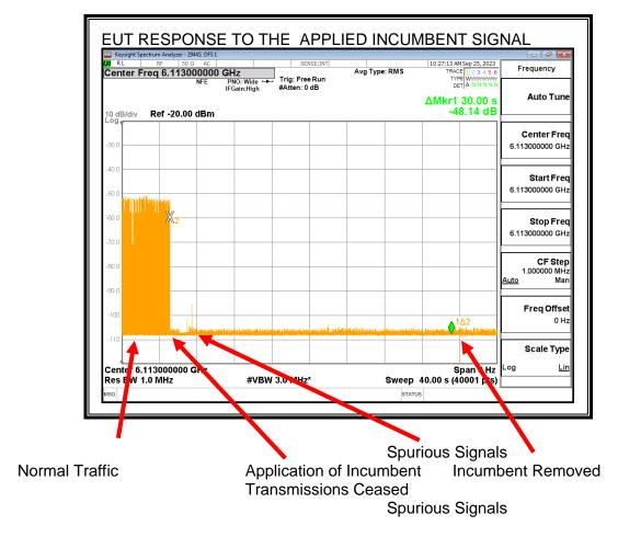
When the EUT detects the Incumbent AWGN Signal it switches channels and all transmissions on the test channel cease.
