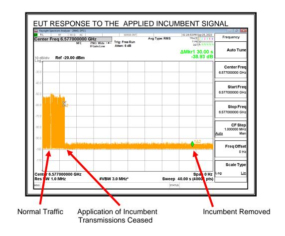
When the EUT detects the Incumbent AWGN Signal it switches to channel 65 and all signals on the test channel cease.
