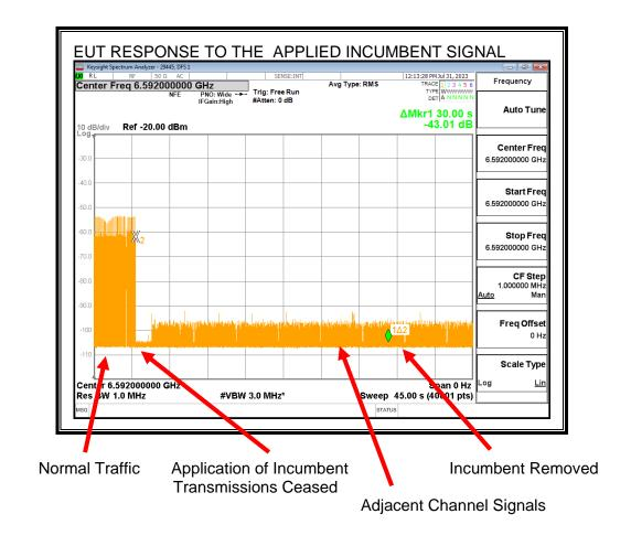
When the EUT detects the Incumbent AWGN Signal it switches to channel 65 and all signals on the test channel cease. Observable transmissions during the monitoring period are from the new adjacent channel to which the EUT has switched.
