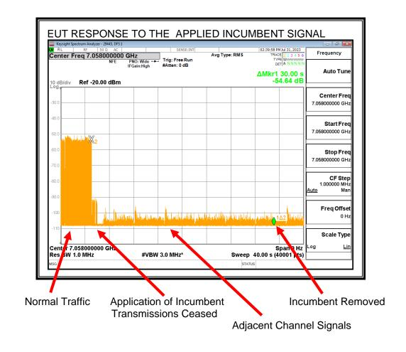
When the EUT detects the Incumbent AWGN Signal it auto-negotiates down to 160 MHz channel bandwidth centered at 6825 MHz. Observable transmissions during the monitoring period are from the 160 MHz adjacent channel.
