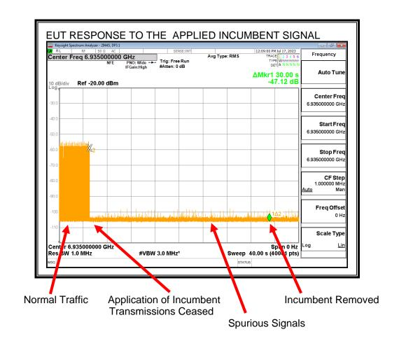
When the EUT detects the Incumbent AWGN Signal it switches channels and all signals with the exception of spurious signals on the test channel cease.
