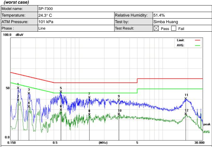
Remark: Factor = Antenna Factor + Cable Loss – Pre-amplifier.
