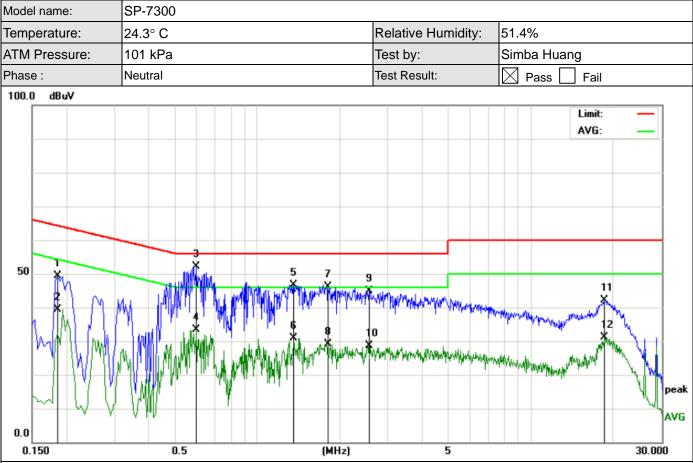
Remark: Factor = Antenna Factor + Cable Loss – Pre-amplifier. Measurement Result=Reading Level +Correct Factor; Over Limit= Measurement Result- Limit;
