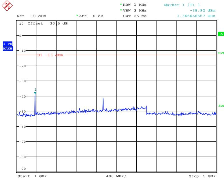
**30MHz – 1 GHz, Channel Spacing 25 kHz, 456.0125 MHz, For FCC part 80**
