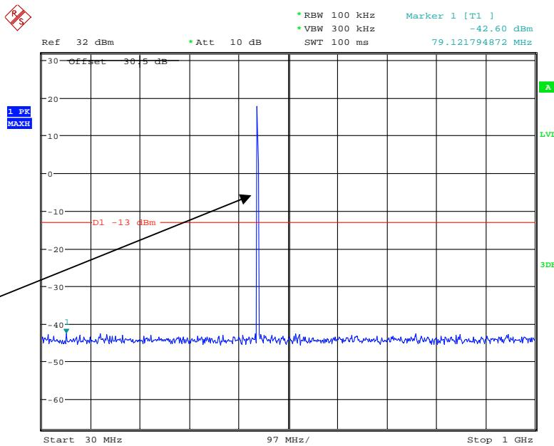
**1 GHz – 5 GHz, Channel Spacing 25 kHz, 454.0125 MHz, For FCC part 22**
