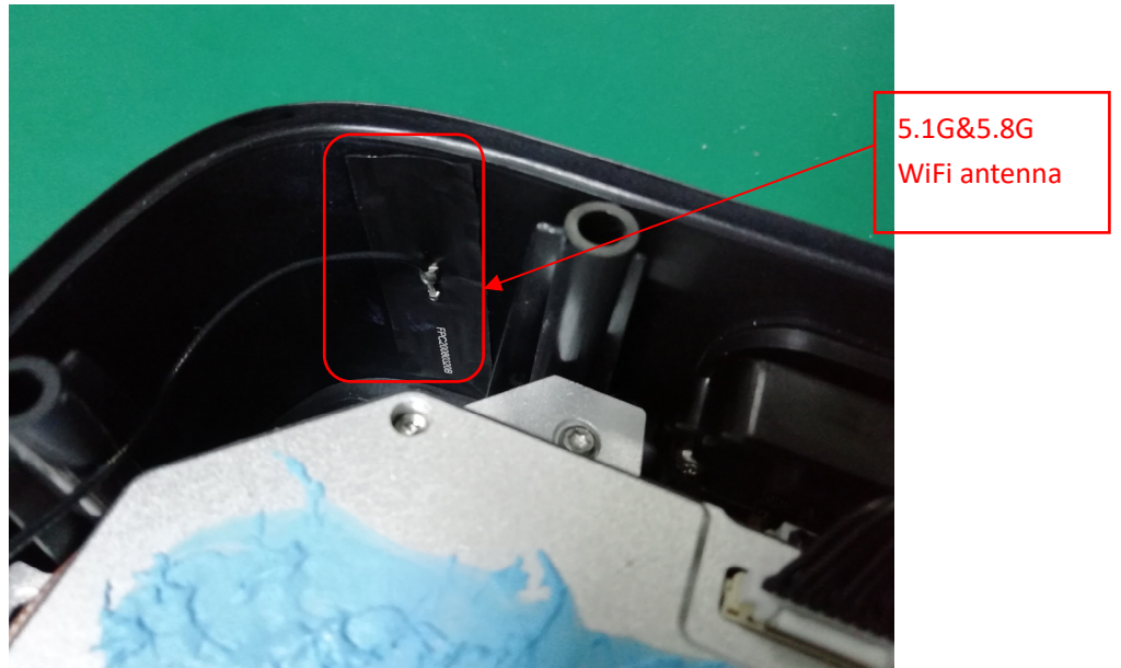
close-up of the 5.1G&5.8G WiFi antenna photo
