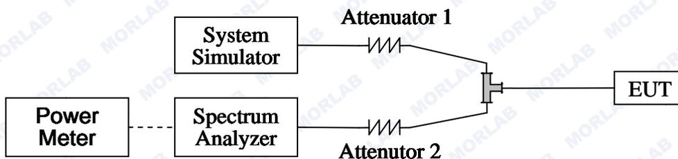
The EUT, which is powered 5V DC power (USB port), is coupled to the Spectrum Analyzer (SA) and the System Simulator (SS) with Attenuators through the Power Splitter; the RF load attached to the EUT antenna terminal is 50Ohm; the path loss as the factor is calibrated to correct the reading. The EUT is commanded by the SS to operate at the maximum output power. A call is established between the EUT and the SS.
