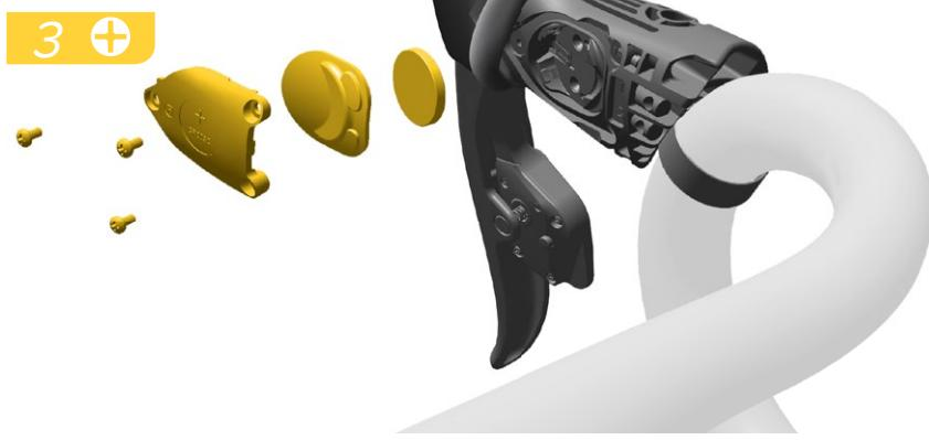
Install a new CR2032 battery with the positive + sign facing outward. Wipe the gasket with a lint-free rag so it is free of dirt and debris, then install the gasket and battery hatch.
