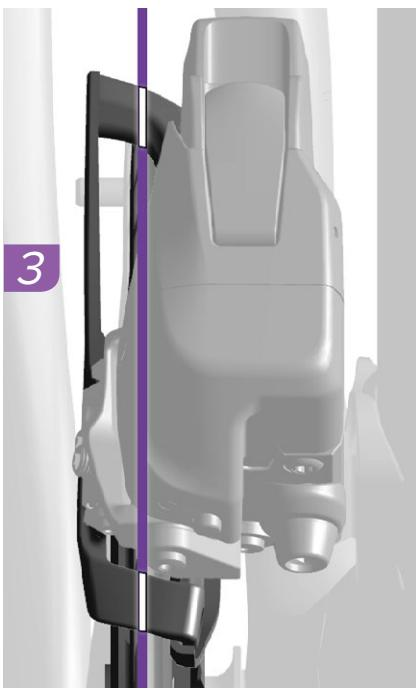
Rotate the front derailleur to align the guide marks on the derailleur to the large chainring.
