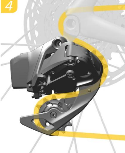
Place the chain onto the smallest cassette cog. Route the chain through the rear derailleur pulleys, and above the tab in the cage.
