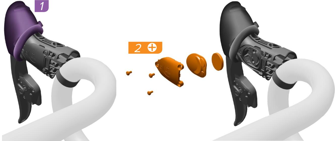
Fold the hood cover forward and remove the three battery hatch screws. Remove the battery cover, gasket, and battery.
