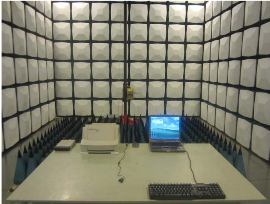
Radiated Emission Above 1GHz -Front View (USB downloading)
