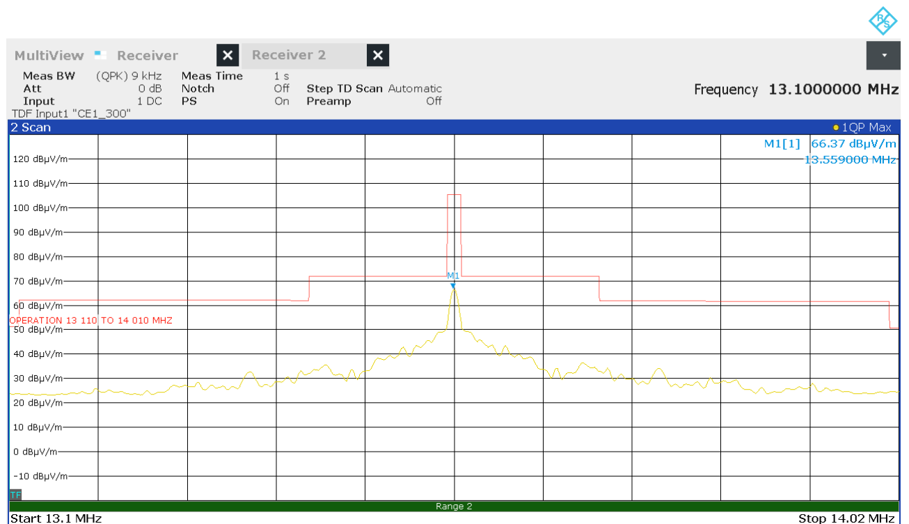
Figure 12: Chart of emission within the band 13.110 MHz to 14.010 MHz, EUT in position Y, without tag, antenna in line at 3 m distance
