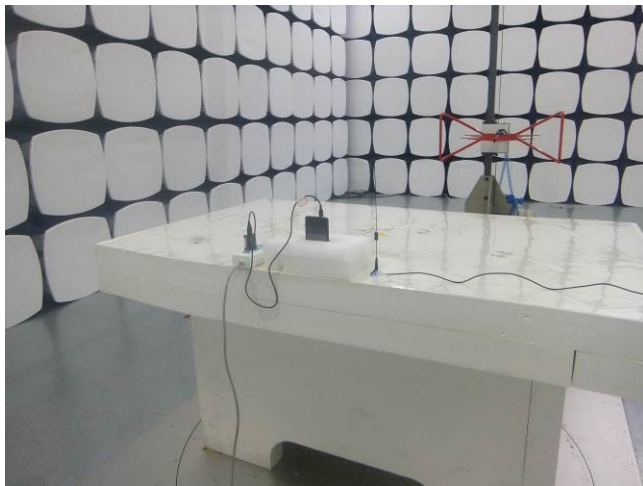
Radiated Spurious Emissions Test Setup Below 1GHz
