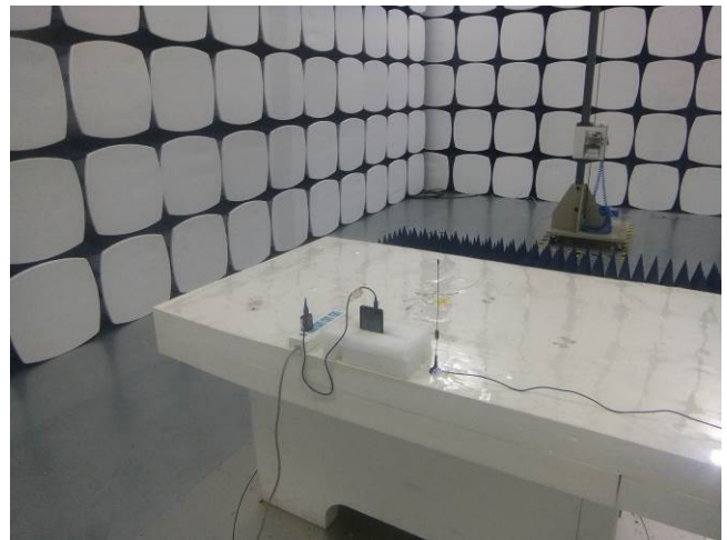
Radiated Spurious Emissions Test Setup Above 1GHz
