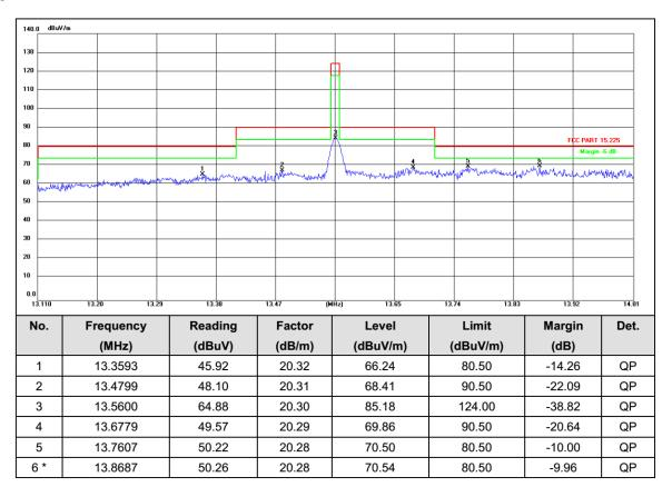
\*Note: Factor= Antenna Factor + Cable Loss
