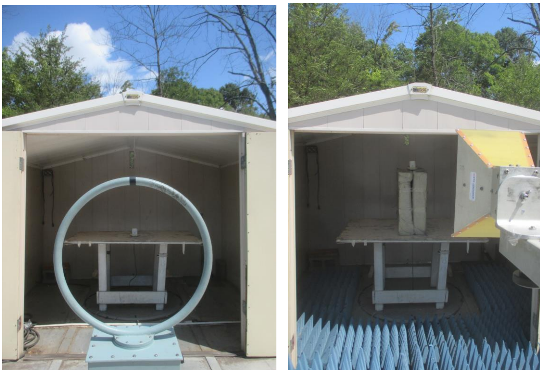
Figure 3.1 Radiated Test Setup
