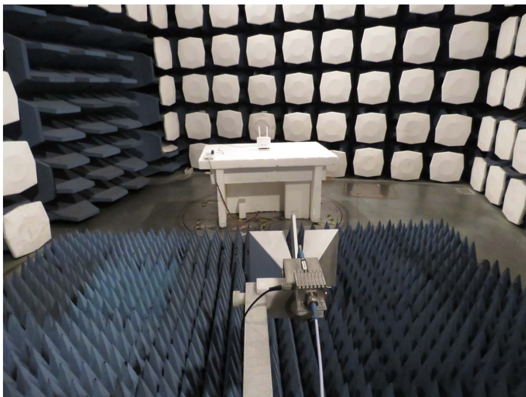
Picture 2: Radiated Spurious Emissions Test setup
