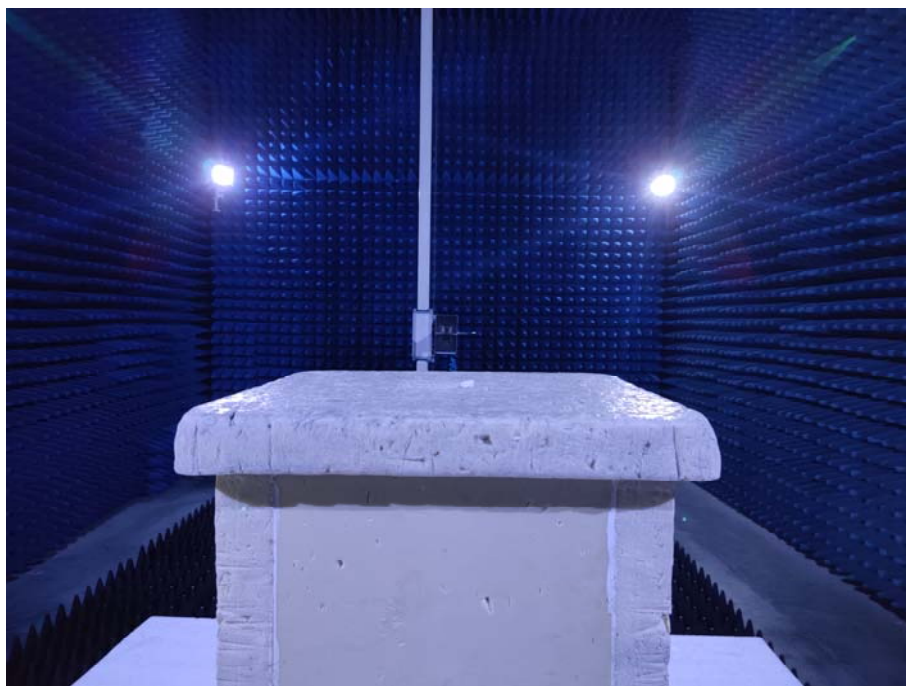
Photo of Radiated Emission Measurement (Above 1G)
