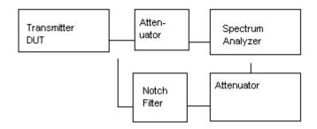
Method of Measuring Conducted Spurious Emissions
