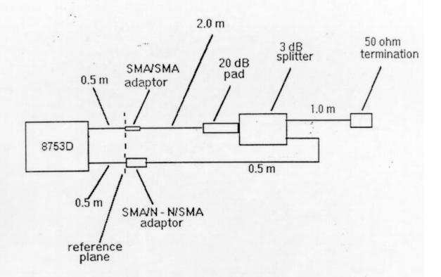
The total loss of this cable assembly from the RF input to the RF output was measured to be 24.40 dB at 815.5 = -3 Mhz.
