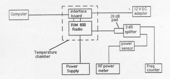
The power supply was adjusted to the required value. The chamber was switched on and the temperature was set to +50°C. After the chamber stabilized at +50°C there was an initial soak period of one hour to ensure that all moisture is driven out. The Radio was switched on and Frequency and power measurements were made as follows:
