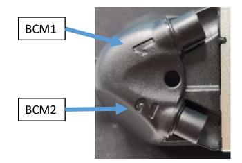
Attach remote or display HMI cable to BCM2
