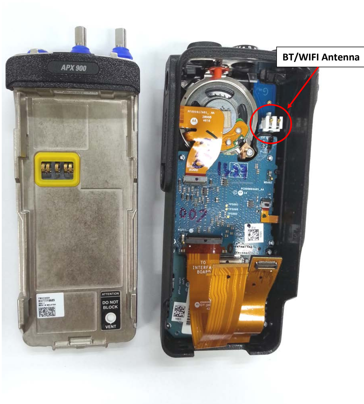
Chassis and Housing (Back), Model 3 (APX900)
