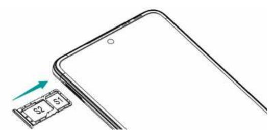
When inserting your card tray, make sure that the card is level and that the card is aligned correctly.
