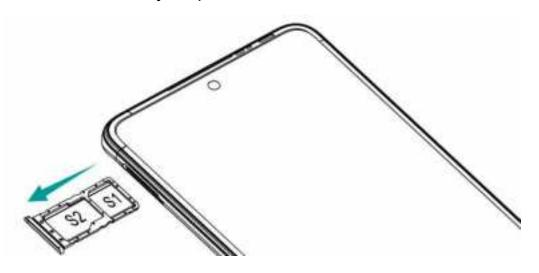
To eject SIM or MicroSD card, insert your SIM eject pin into the small hole next to the card tray.
