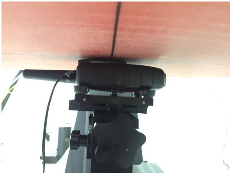
**Body-worn, the rear of the EUT towards ground with A1, B1, BC1 and AC1**
