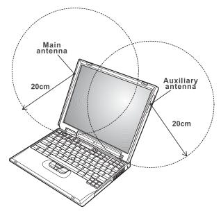
**Note:** IBM Dual-Band 11a/b Wi-Fi Wireless Mini PCI Adapter implements transmission diversity function. The function does not emit radio frequencies simultaneously from both antennas. One of the antennas is selected automatically or manually (by users) to have good quality of radiocommunication.
