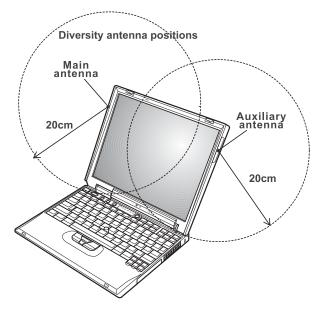
**Note:** The transmission diversity function is implemented for the Card (FCC ID: ANOU58H004). The function does not emit radio frequencies simultaneously from both antennas. One of the antennas is selected automatically or manually (by users) to have good quality of radiocommunication.
