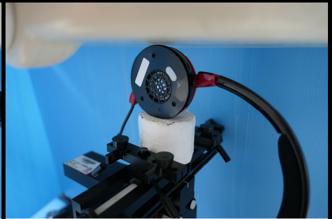
Rear Face of Earphone Tested at 0 mm
